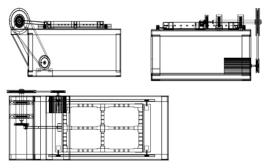
Figure 1. The orthographic projection of the globulator
